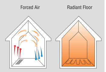
Unlike forced-air systems, radiant heat stays near the floor, not the ceiling, creating an even, consistent heat.
