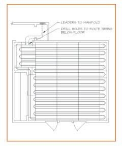
Comfort Track™ is a modular radiant flooring system that is composed of medium density composite wood, covered with an aluminum adhesive. The aluminum accelerates the heat transfer from the tubing to the flooring. The boards can accept Embassy's 3/8" Liquipex<sup>™</sup> tubing, as well as any 3/8" PEX tubing that is manufactured to ASTM F876. Each board is grooved, which keeps the PEX tubing securely in place. This "tight fit" ensures excellent and rapid thermal transfer to the finished floor.
