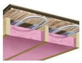
extruded snap plates, peak performance is assured. For less demanding requirements the tubing can be affixed to the subfloor using customfitted staples and or reflector snap plates.
