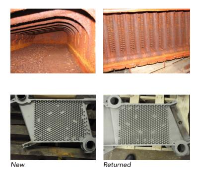
Areas that were expected to have the highest levels of wear were cut down even further for a more detailed examination. The areas exhibiting the most corrosion were then milled until the surface was free from pits and revealed clean cast iron. Together, the weight of the removed castings and the extent of surface pitting indicate a 1 - 2% loss of cast iron throughout Boiler 1 and 2's lifecycles.
