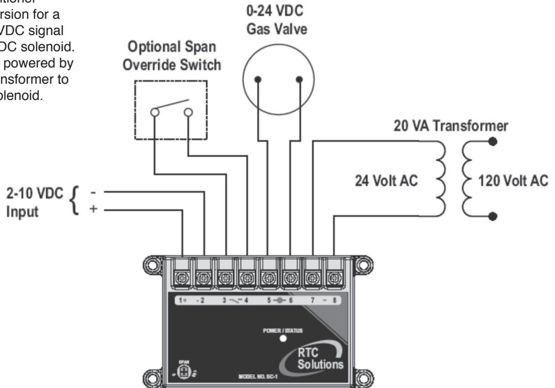
*Span Override Switch* - When terminals 3 & 4 are shorted together the span setting is ignored forcing the ratio to 100%.
