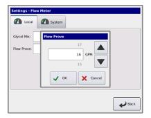
When the boiler has a heat demand it will not start until the programmed GPM requirement is met. If the boiler is running, it will also stop firing when the GPM falls below the Flow Prove value. In this case the minimum flow is below the required 16 GPM so the boiler will not start. The flow proof time has expired and then enters into a fault condition.
