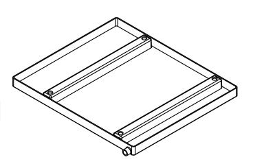
SpacePak has designed a series of secondary drain pans specifically sized for use with all horizontal fan coil units. Exclusive built-in supports raise the unit off the bottom of the drain pan. Installed with threaded rod, the unique pan construction fully supports the fan coil unit. For use with all ESP or WCSP series coil units.
