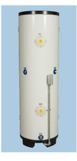
As a hydraulic separator, BT's separate the hydronic from the energy source loop (heat pump / boiler) from the hydronic flow in the distribution system (air handlers / emitters). Hydraulic separation is used primarily in systems where flow rates from the source to the distribution vary or with applications utilizing variable speed pumps. The heating or cooling source can be hydraulically decoupled from the distribution system.
