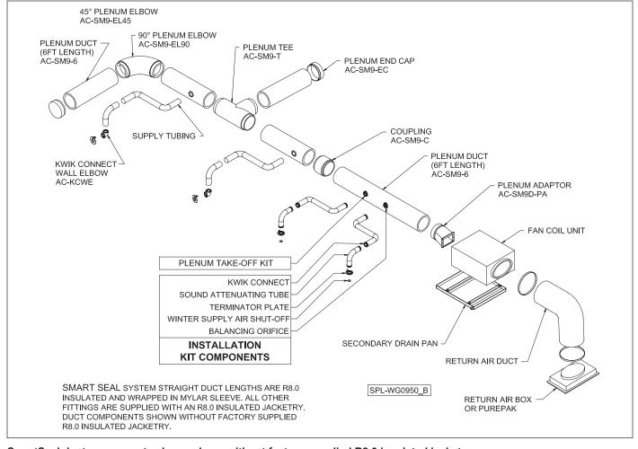
SmartSeal duct components shown above without factory supplied R8.0 insulated jacketry.
