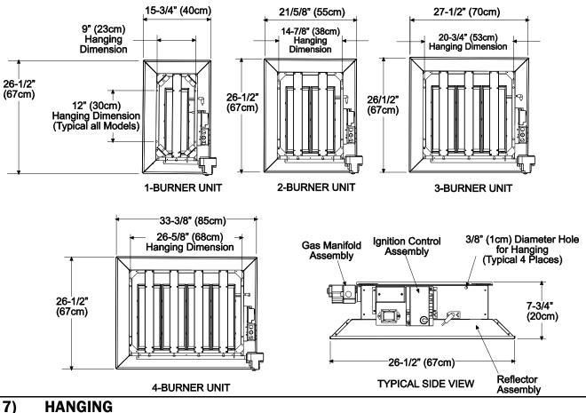
Always suspend from a permanent part of the building structure that can support the total force and weight of the heater.
