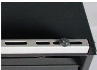
The flush mount hanger arm is slotted to receive a 5/16" lag bolt 16" or 24" on center. It can be attached parallel or perpendicular to the joist.
